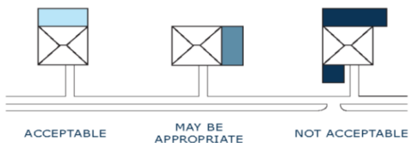
Figure 96: Diagram of appropriate and inappropriate locations of additions.
