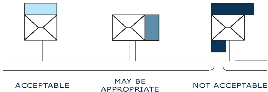
Figure 107: Diagram of appropriate and inappropriate locations of additions.
