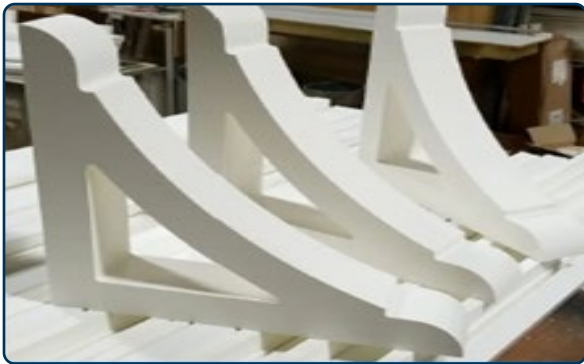
Figure 122: Substitute material brackets (Source: Executive Architectural Millwork).
