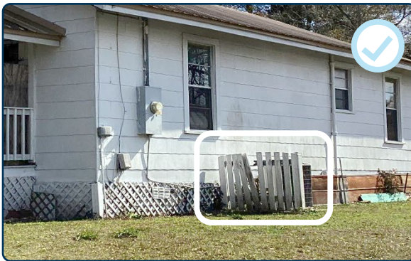
Figure 90: An appropriate location for the installation of an HVAC system that is near the rear of the residence and screened behind fencing.
