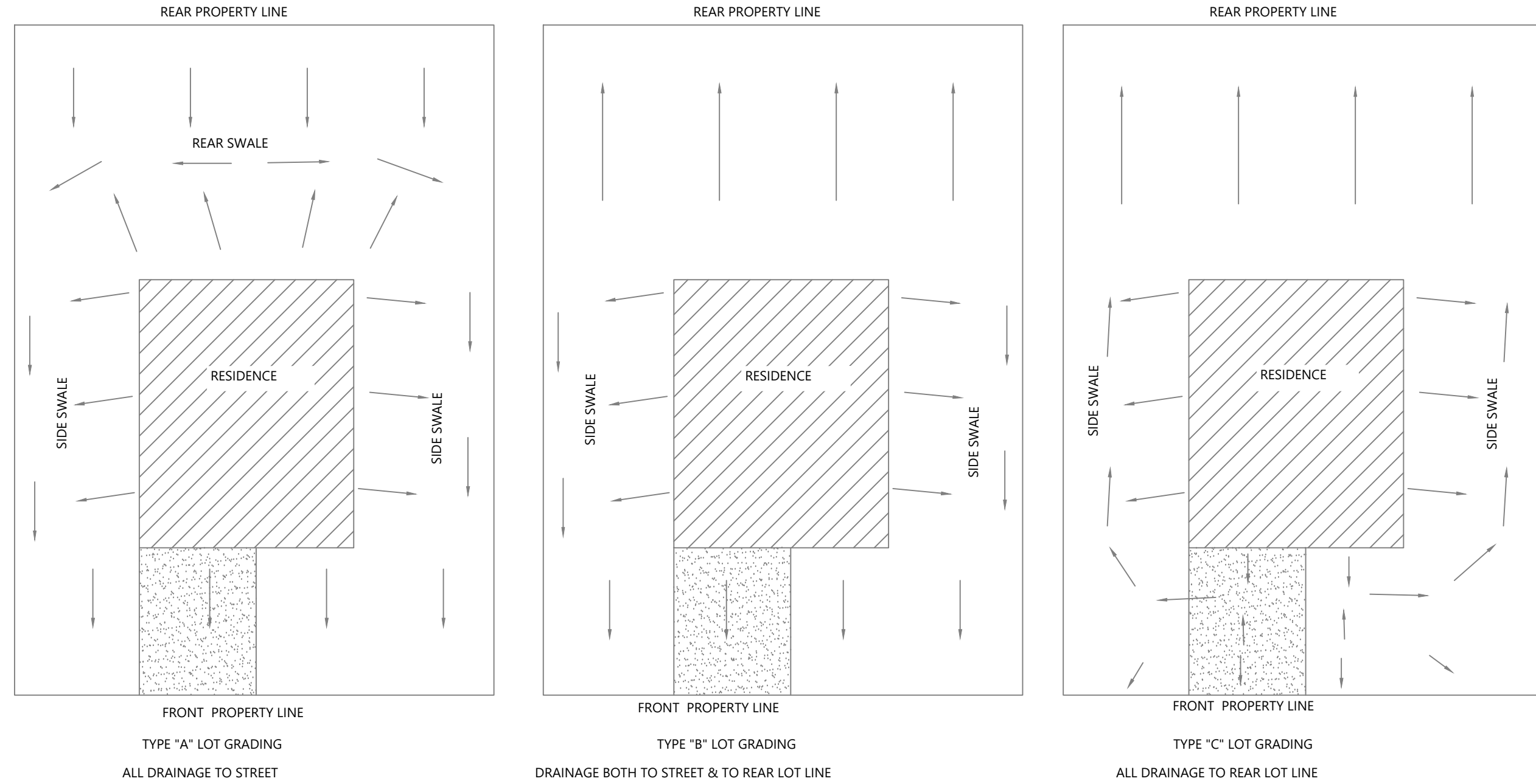
2 TYPICAL LOT GRADING (C8.1) SCALE: N.T.S.
